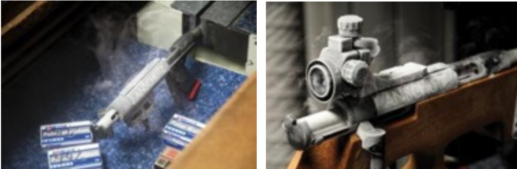
Pictures : Shooting tests in the cold chamber of Anschütz company at -30°C
