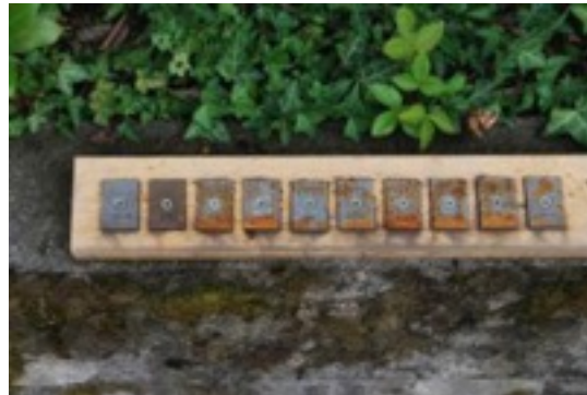
1=CERACOAT gun coating, 2=Gunex, 3=Remington, 4=Ballistol, 5=Liqui Moly Guntec, 6=Motorex Guncare , 7=Steel ST37 8=Brunox, 9=Neoval, 10=WD40
